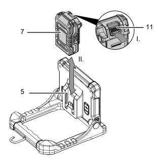
2. If required, charge the battery (7) as described in the section *Charging the battery*.
